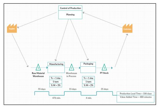
Figure 2. Value Stream Mapping (VSM)
