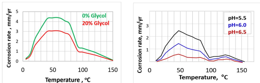
**Figure 1: Effect of glycol on corrosion rate** **Figure 2: Effect of pH on corrosion rate**
