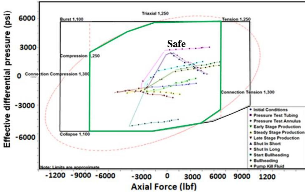
Figure 8: All loading within the safe design limit (green curve) for unworn tube
