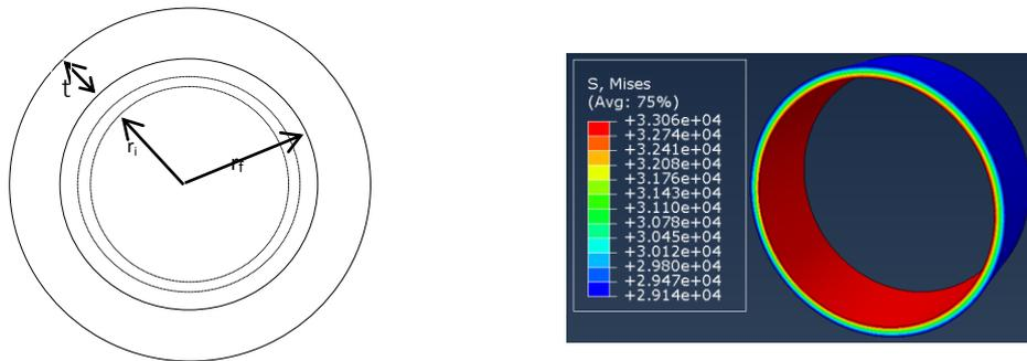
Figure 3 Inner surface uniformly removed tube    Figure 4: von Mises stress field
