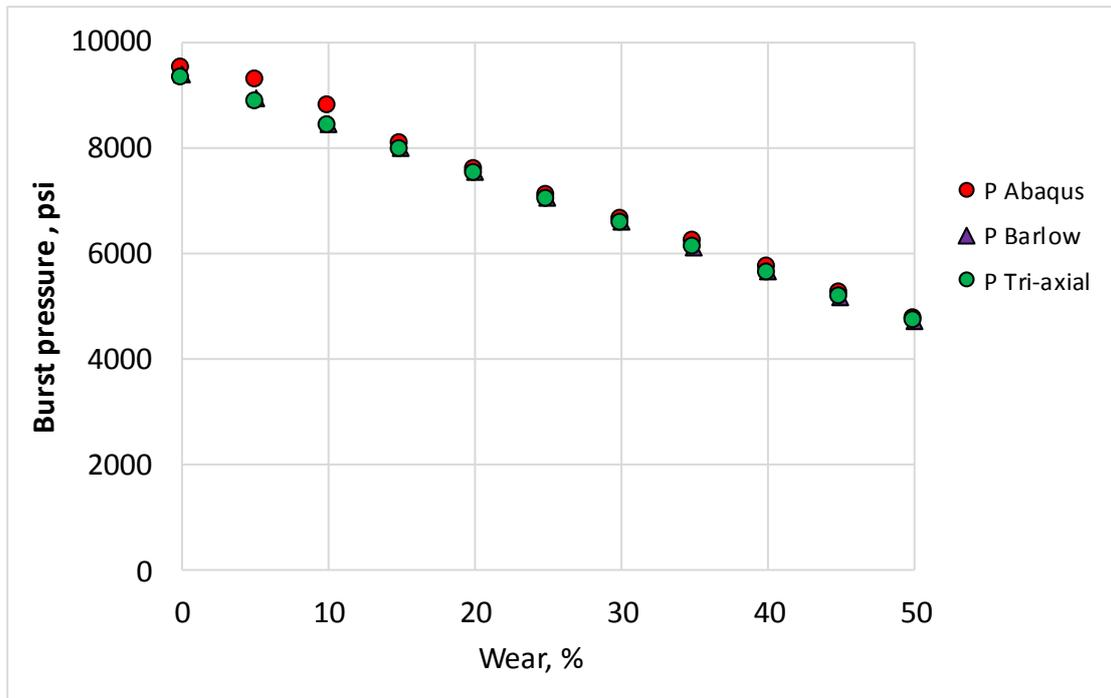
**Figure 6: Simulation vs. theoretical burst de-rated pressures.**
