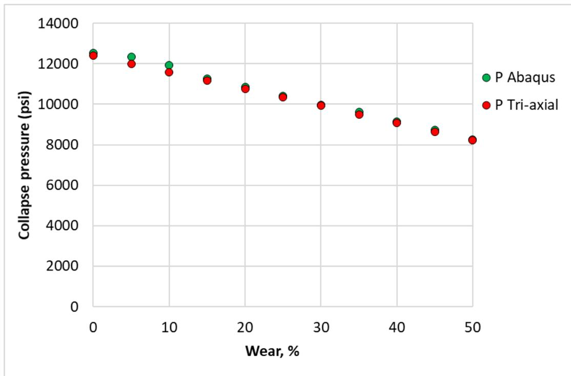
**Figure 7: Simulation vs. theoretical collapse de-rated pressures**
