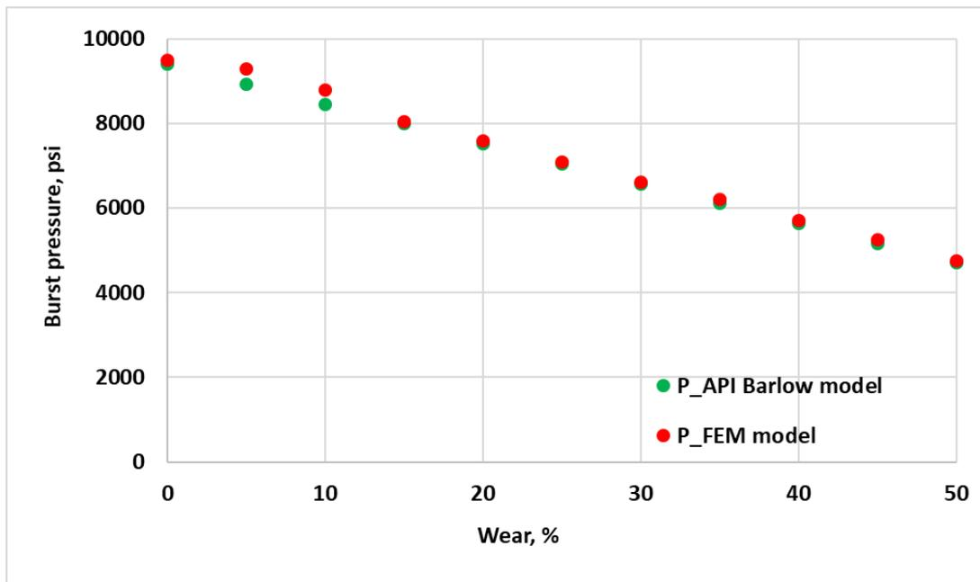
Figure 5: Comparisons between burst de-rating API Barlow and EFM modeling.
