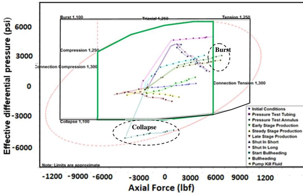
Figure 9: Three loads crossing design limit for tubing with 20% worn out
