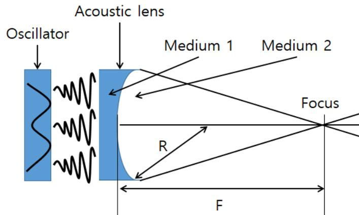
Fig 2. Schematic of Acoustic Lens
