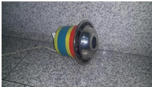
**Fig 1.** Portable Sound Fire Extinguisher
