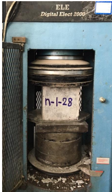
Fig.1 Compressive strength test setup
