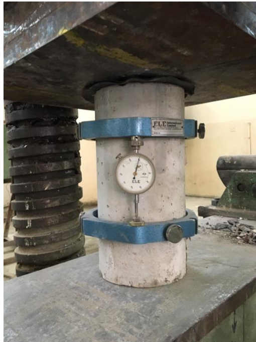
Fig.3 Modulus of elasticity test setup
