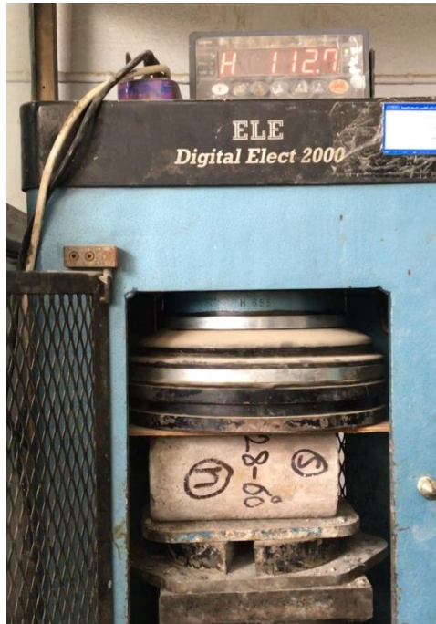
Fig. 4 Tensile strength test setup
