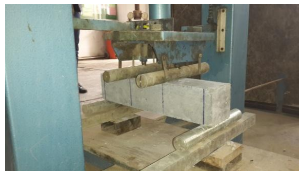
Fig.2 Modulus of rupture test setup
