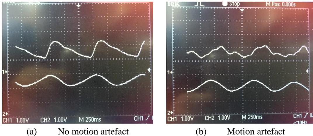
**Figure 5.** An IIR BPF output (lower wave) for the detection of NNI based on the PPG signal (upper wave) and the impact of a motion artefact.
