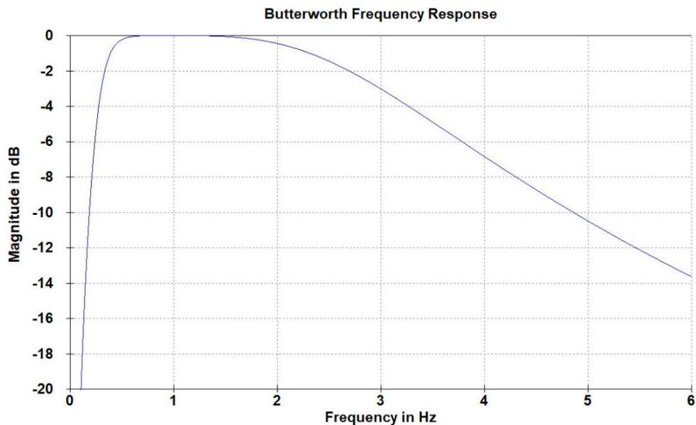
**Figure 4.** Magnitude frequency response of digital IIR BPF with -3 dB at the desired second cutoff frequency  $f_{d2} = 3$  Hz.
