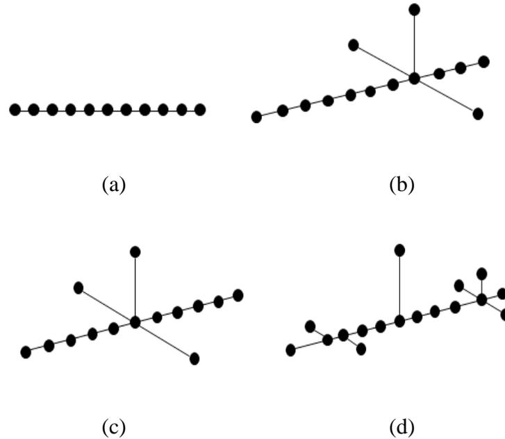
**Fig.2** 3D highlight models of targets for synthesis of active sonar signals.
