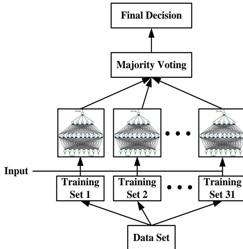
**Fig. 3** Structure of classifier ensemble for the experiment
