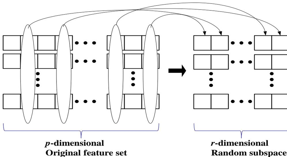
**Fig. 1** Resampling method in feature space in RSM
