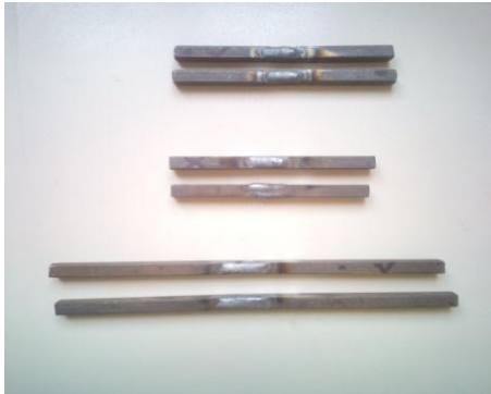
Figure.6 Sample after welding
