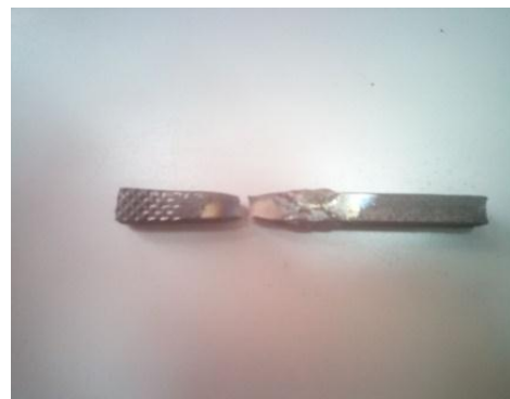
Figure .9. Sample after tensile test
