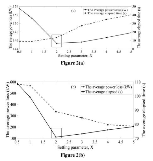
Figure 2. The average power loss and elapsed time of 33 bus system as a function of setting parameter X of SSA for (a) the system reconfiguration and (b) the capacitor placement problem.
