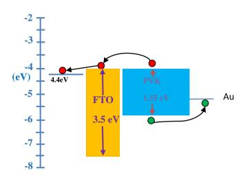
**Fig.1(b).** Energy band diagram of device (Perovskite is shown as PVK).
