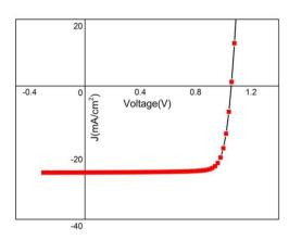
**Fig. 4. (a)** J-V curve for optimum perovskite absorber thickness of 2.3 μm.
