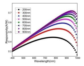
Fig.10. Responsivity variation with wavelength for different values of perovskite absorber thickness.
