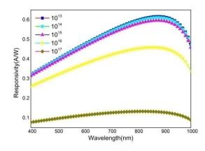
Fig.11. Responsivity variation with wavelength for different values of bulk defect density.
