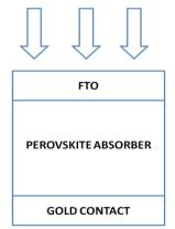
Fig.1(a). Perovskite device structure.
