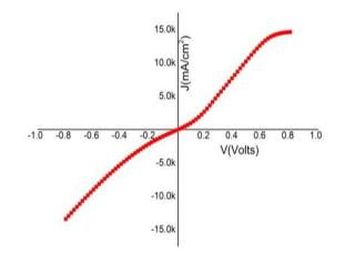
**Fig. 3.** J-V characteristic of Perovskite solar cell with Silver as back electrode.
