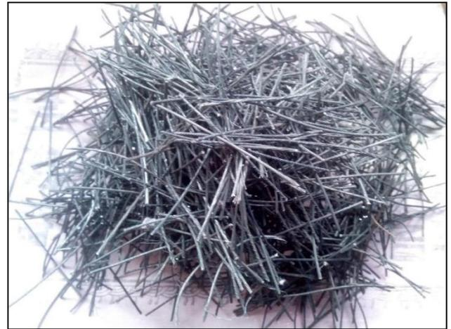
**Fig. 1.** Recycled tyre steel fibre
