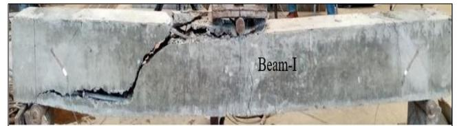
Fig. 8. Crack and failure pattern of Beam-I
