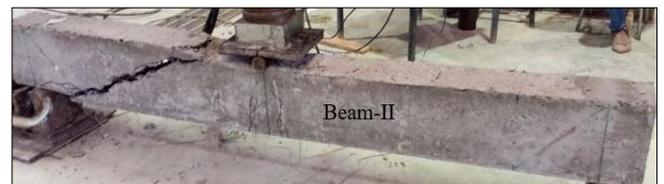
Fig. 9. Crack and failure pattern of Beam-II
