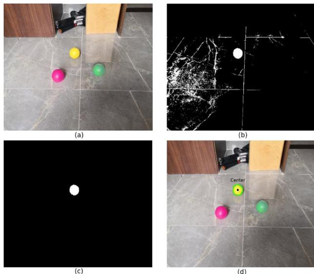
**Fig. 2.** Operation of the algorithm in the laboratory. (a) The three balls used for evaluation: yellow, green and red. (b) Image binarized by HSV color space. (c) Identification of regions by morphological adjustment, and (d) Initial image with superimposed localization information
