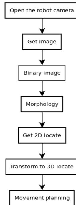
**Fig. 1.** Functional description of the identification algorithm
