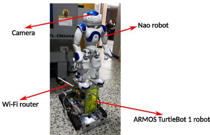
**Fig. 3.** Experimental setup for the identification system. It is composed of a humanoid Nao robot from SoftBank Group at the top and an ARMOS TurtleBot 1 tank robot from the ARMOS research group at the bottom
