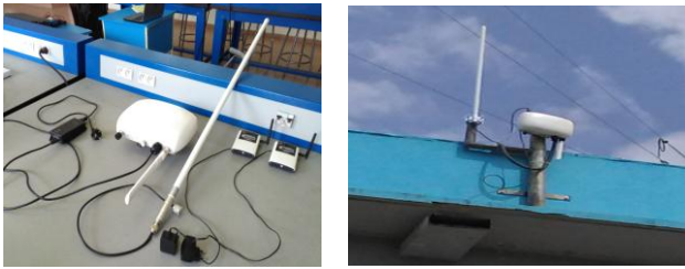
Figure 3: ESATIC LoRa base station
