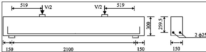
Fig. 6. Dimensions of the beams in (mm)
