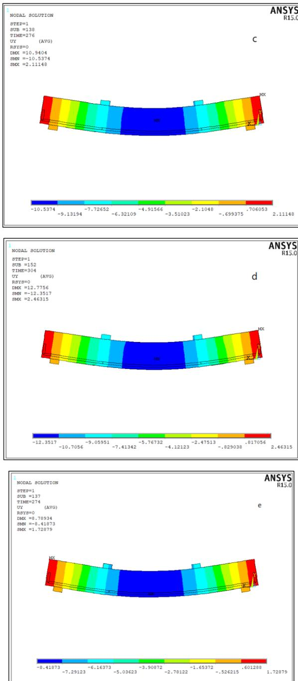
**Fig. 12.** The variation of displacement along the beams a) B00, b) B0.5, c) B1.0, d) B1.5 and e) B2.0) at ultimate shear force.
