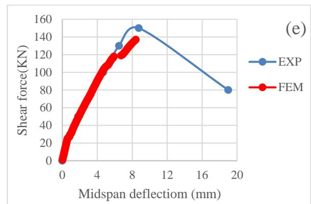
**Fig. 9.** Shear force-midspan deflection for a) B00, b) B0.5, c) B1.0, d) B1.5 and e) B2.0
