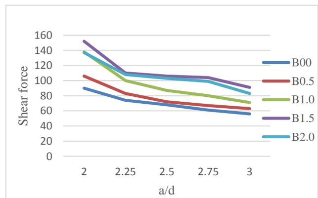
**Fig. 14.** Shear force-shear span to depth ratio relations for the beams
