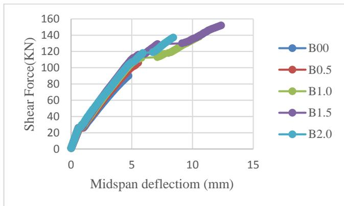
**Fig. 10.** shear force-midspan deflection curves of the SFRC beams
