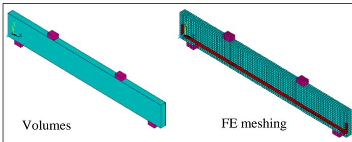
Fig. 7. (FE) modelling of the beam
