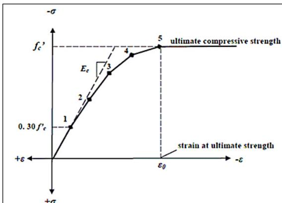
**Fig. 1.** Uniaxial stress-strain curve for concrete in compression
