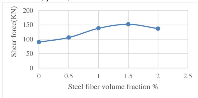
**Fig. 11.** Relationship of shear force and steel fiber volume fraction.
