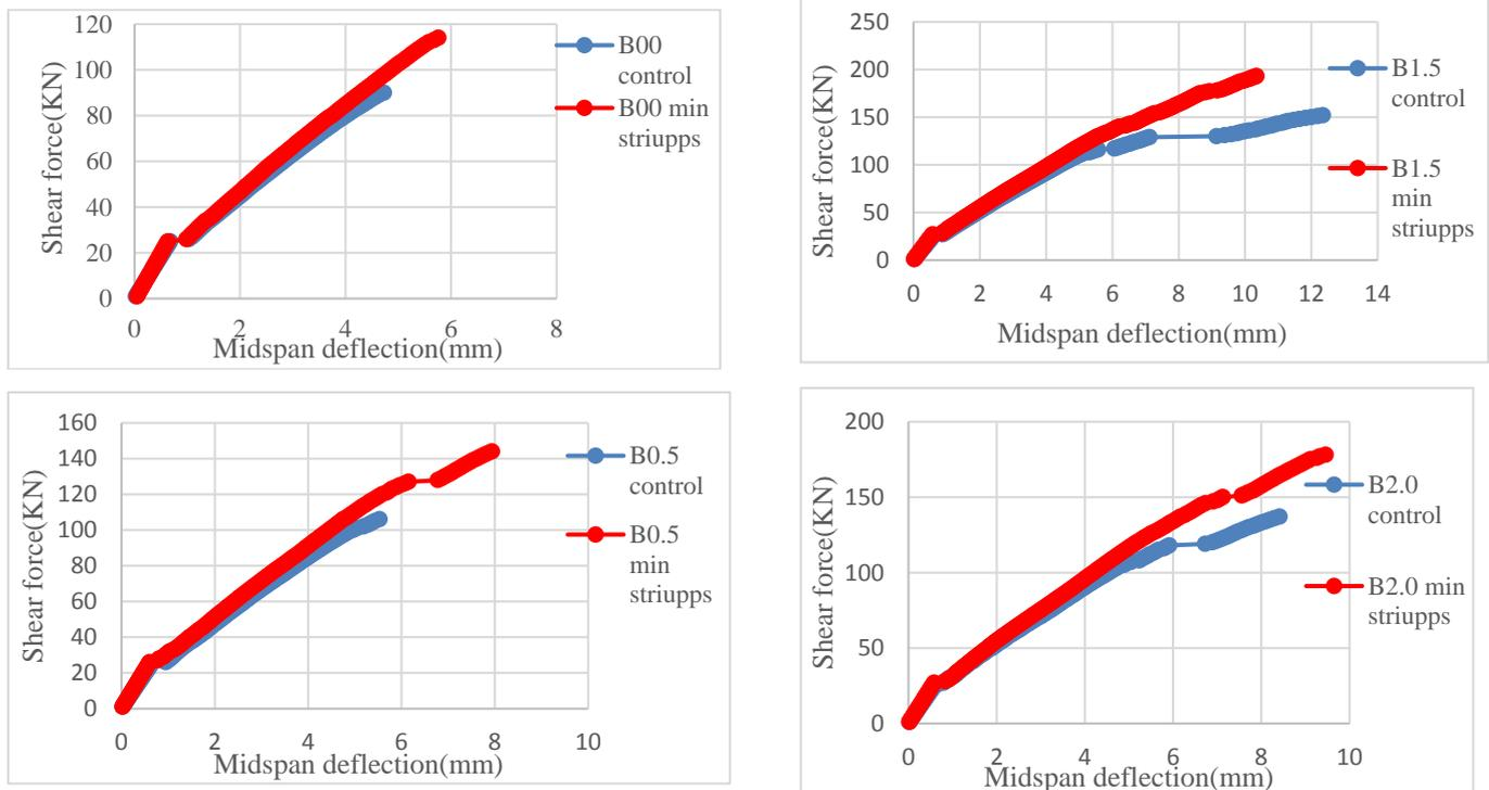
**Fig. 15.** Shear force-deflections curves of the beams with minimum shear reinforcement.
