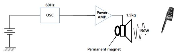
Fig 4. Output measurement using general permanent-magnet type speaker
