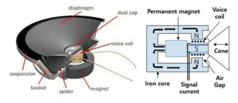
Fig 2. Structure of permanent-magnet type speaker [http://www.audiocircuit.com/][7]
