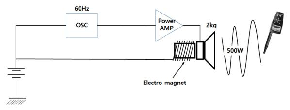
Fig 5. Output measurement using an improved electro-magnet type speaker
