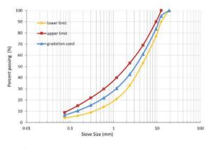
Fig 1. The Gradation of Aggregate (AC-WC)
