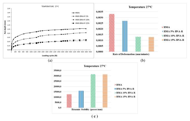
Fig. 7. WTM Result at Temperature of 27 °C
