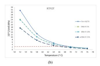
**Fig 6.** The Change of G\*/sinδ (anti rutting factor)
