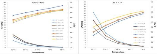
**Fig. 2**. Change of  $G^*$  and  $\delta$  at the Temperature Sweep
