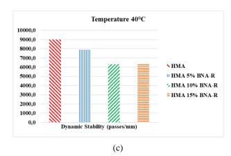
Fig. 8. WTM Result at Temperature of 40°C
