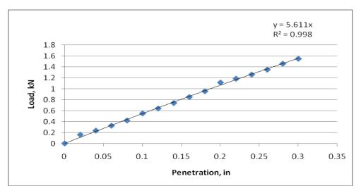
Fig. 8. CBR results of contaminated soil sample having 5% engine oil
