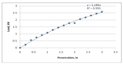
Fig. 7. CBR results of reference soil specimen .
