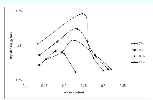
Fig 3. Density-moisture relationships of the reference and contaminated soil samples.
