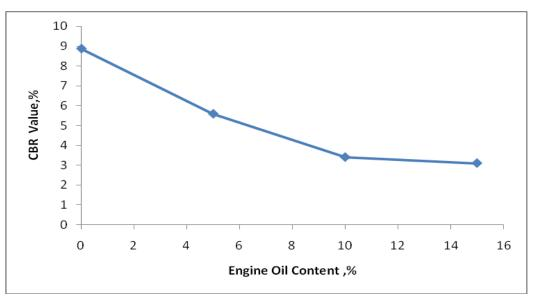
Fig.11. The CBR values of the reference and contaminated soil specimens.
