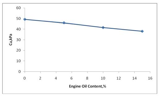
Fig. 5. Effect of engine oil dosage on unconfined compressive strength .
