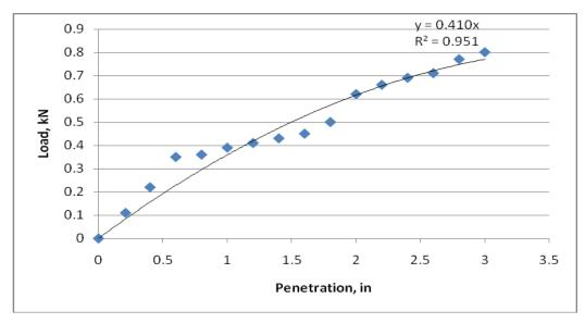
Fig. 10. CBR values of contaminated soil sample having 15% engine oil .
