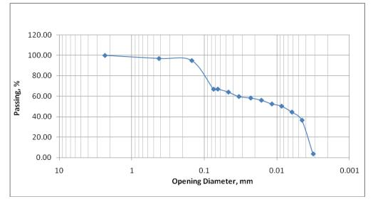
Fig 1. Grain size distribution of soil used
