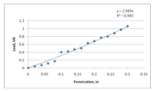
Fig. 9. CBR results of contaminated soil sample having 10% engine oil .
