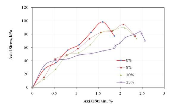
Fig. 4. Unconfined compression tests of reference and contaminated soil specimens.
