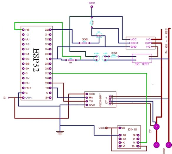
Fig 3. Schematic design of smart socket module.
