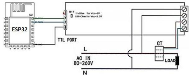
Fig 2. Connection of PZEM-004T and ESP32 unit
