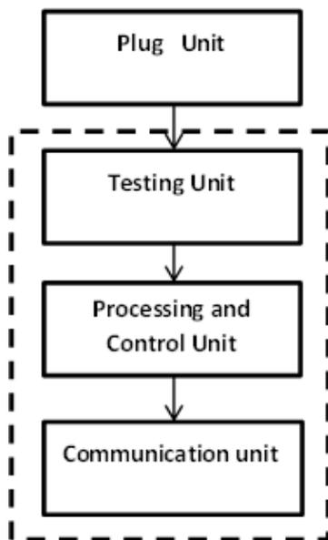
Fig 1. Diagram of smart socket
