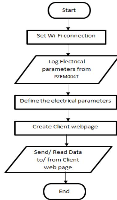
**Fig5.** Flowchart for software programming
