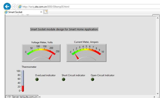
**Figure 6.** Monitor of electrical parameters
