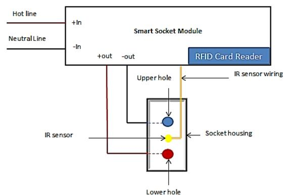
Fig. 4. The electrical connection of smart socket module for two holes of standard socket.
