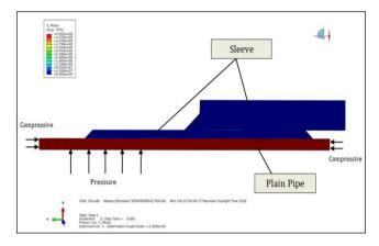
Figure 4:Initial States - Preloaded Plain Pipe (Von Mises: Pa)
