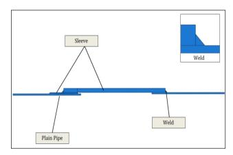
Figure 1: Model – Sleeve Assembly
