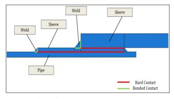
Figure 3: Contacts – Sleeve Assembly
