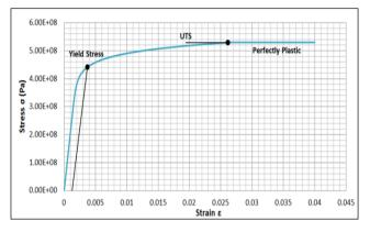
Figure 2: Elastic-Plastic Curve – CSA Z245.1 Grade 448
