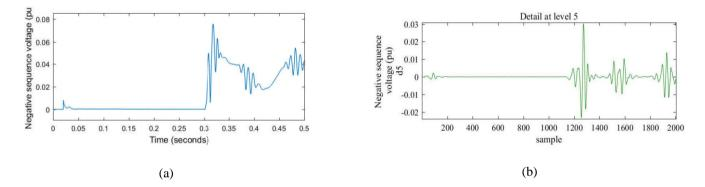
Fig. 5. (a) Negative sequence component of voltage during islanding condition, (b) DWT at level 5
