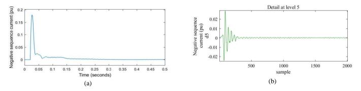
Fig. 4. (a) Negative sequence component of current during normal operation, (b) DWT at level 5
