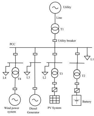
Fig. 2: Grid-connected microgrid
