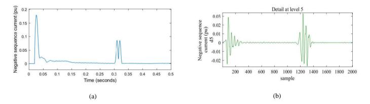
Fig. 6. (a) Negative sequence component of current during islanding condition, (b) DWT at level 5
