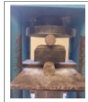
Fig. 3: Tensile splitting strength test setup
