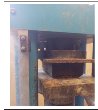
Fig. 2: Compressive strength test setup
