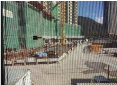
**Fig. 2.** Visual effect of an a-Si PV module with 20% transmittance from inside to outside [11].
