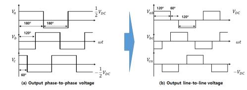
Fig 6. Output of pseudo sinusoidal wave by FET inverter
