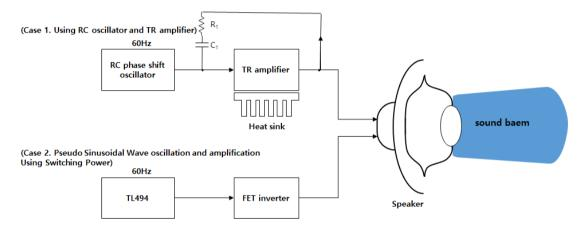
Fig 8. Configuration of the Sound Fire Extinguisher used in the experiment
