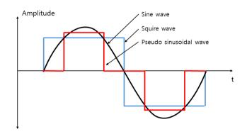
Fig 4. Pseudo sinusoidal wave
