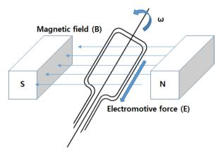
Fig 2. Principles of AC generator [10]
