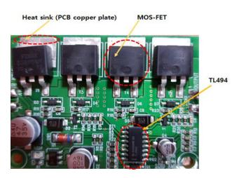
Fig 9. FET pulsed pseudo sinusoidal wave oscillator, amplifier
