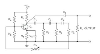
Fig 3. RC phase shift oscillator [11]
