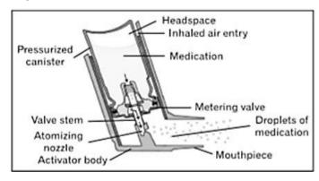
Figure 1. Diagram of the pressurtzed metered-dose inhaler [29]
