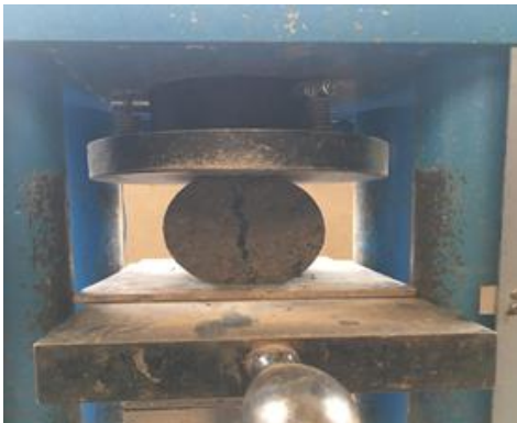
Figure 4. Crushing of specimens
