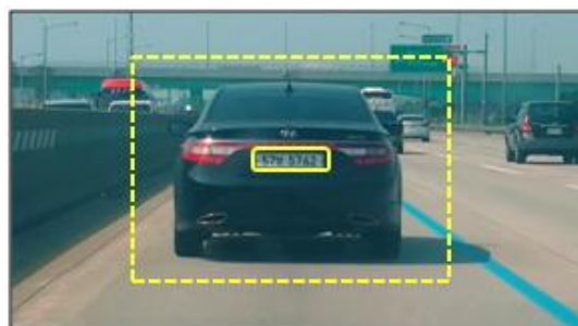
Fig. 10. Specified Area on the Input Image. (Dotted Line: License Plate Tracking Area, Solid Line: License Plate Region of the Vehicle)
