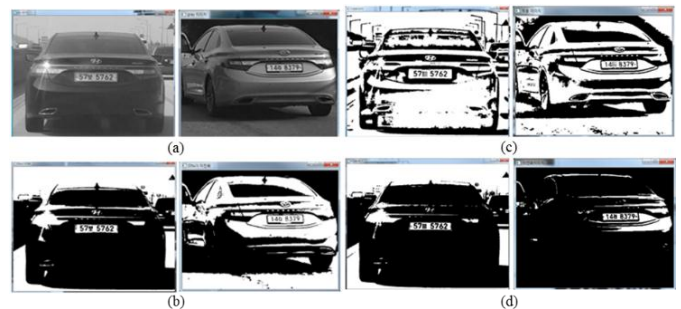
Fig. 15. Results of binarization method, (a) Image area of the license plate tracking region, (b) Results of Otsu's binarization, (c) Results of adaptive binarization, (d) Results of binarization (Thresholding value=140)
