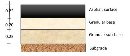
Fig. 2. Structural model for design
