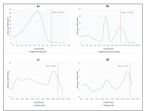
Fig. 1. Load spectrum for: a) single steering axle, b) single axle non-steering, c) Tandem Axle and d) Tridem axle
