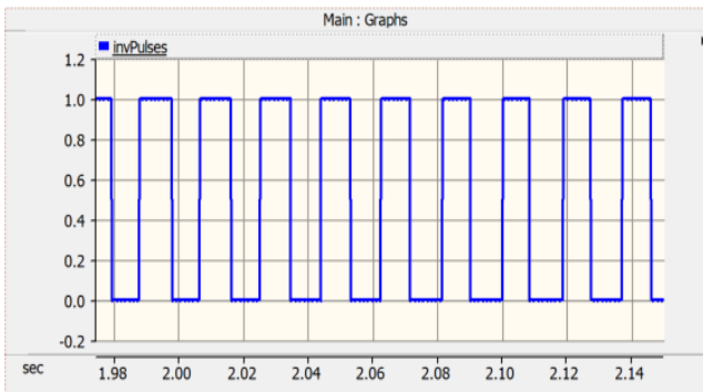
Figure 12: Pulse waveform for firing angles of thyristor
