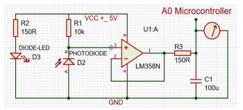
Figure 3. Schematic diagram of a cholesterol monitoring system
