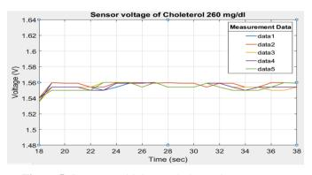
Figure 5. Sensor sensitivity on cholesterol measurement compared to invasive techniques
