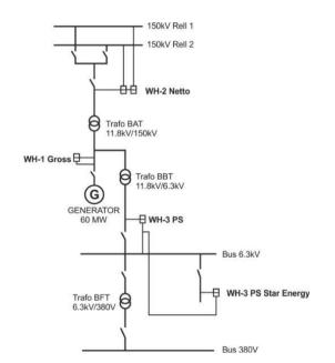
Figure 2. The point of measuring the power on the generator uses a power meter
