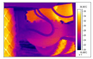
Figure 1. Thermal map of the intermediate axle in the KAMAZ vehicle
