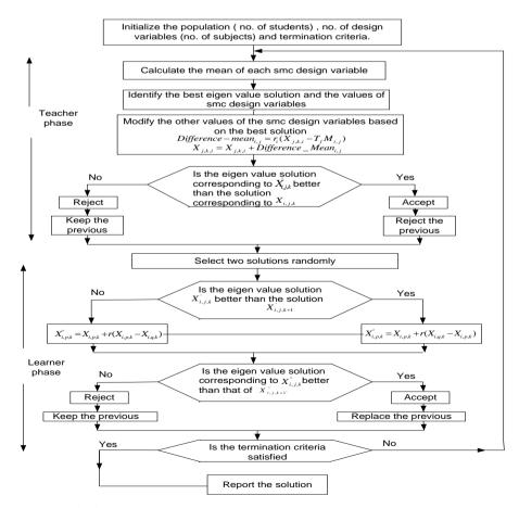
Fig 3: Flow chart for computing optimal values of SMC parameters
