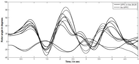
Fig. 10: Plot of rotor angle of generators 1-5 for a 3-phase fault at bus no. 26.
