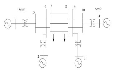
Fig. 5: Single line diagram of 4-machine 2-area system.
