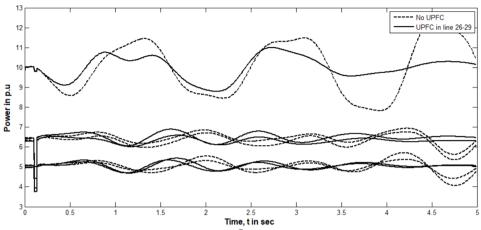
Fig. 13: Plot of real power of generators 1-5 for a 3-phase fault at bus no. 26.
