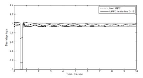
Fig 7: Plot of terminal voltages of generators 1-4 for a 3-phase fault at bus no. 7.
