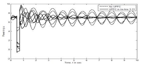
Fig 8: Plot of real power of generators 1-4 for a 3-phase fault at bus no. 7.
