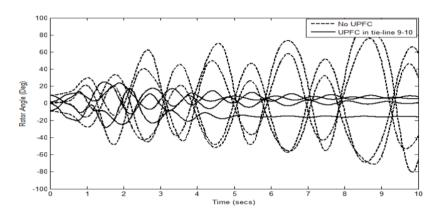
Fig. 6: Plot of rotor angles of generators 1-4 for a 3-phase fault at bus no. 7.
