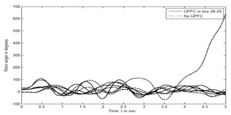
Fig. 11: Plot of rotor angle of generators 6-10 for a 3-phase fault at bus no. 26.
