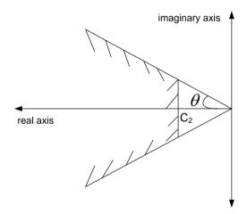
Fig 2 Permissible region for location of closed loop eigenvalues in the left half plane.
