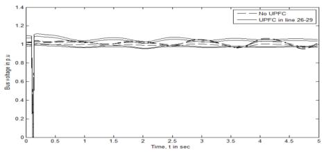
Fig. 12: Plot of terminal voltages at buses 26, 27, 28, 29 for a 3-phase fault at bus no. 26
