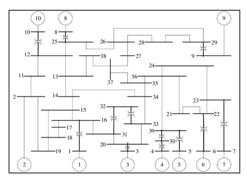
Fig. 9: Single line diagram of 10-machine 39-bus New England system.
