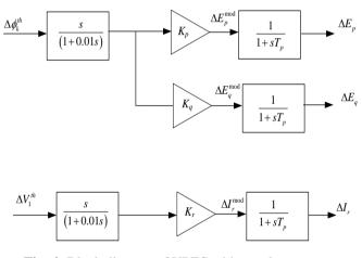
Fig. 4: Block diagram of UPFC with supplementary modulation controllers
