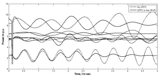
Fig. 14: Plot of real power of generators 6-10 for a 3-phase fault at bus no. 26.
