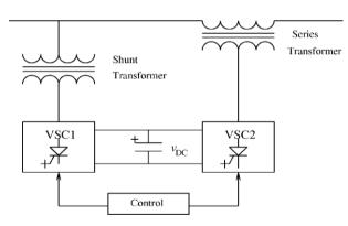
Fig. 1. Unified power flow controller.
