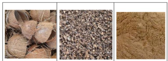
Figure 6: Raw coconut shells, crushed coconut shells and coconut shell powder
