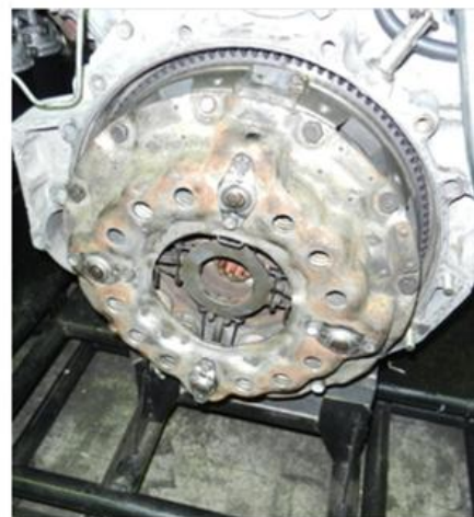
Figure 1. Clutch Assembly of the KAMAZ car (model 142):
