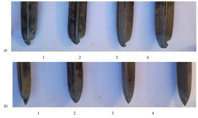
Figure 4. Overall view of tooth points wear after abrasive action according to the presented groups: a - side view; b - front view.
