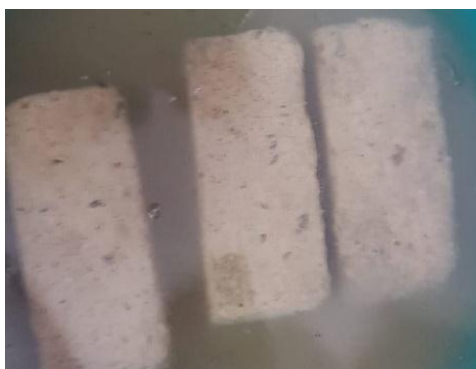
Fig 5: Air cured Bricks after being submerged in acid for 24 hours. (Reaction with Acid test.)
