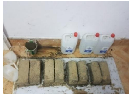
Fig 4: De-moulded, casted bricks.
