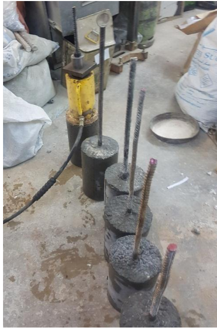
Figure 6. Cylinder in its center with a steel bar undergoing pull-out test
