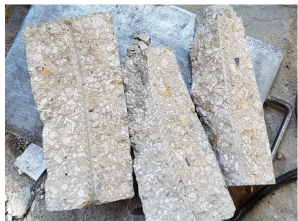
Figure 7. Used after segmentation deformed steel bar indentations
