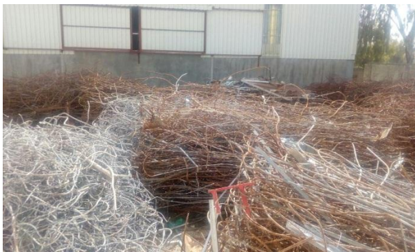
Figure 3. Recycled steel bars arrive in the industrial area of Rageeb
