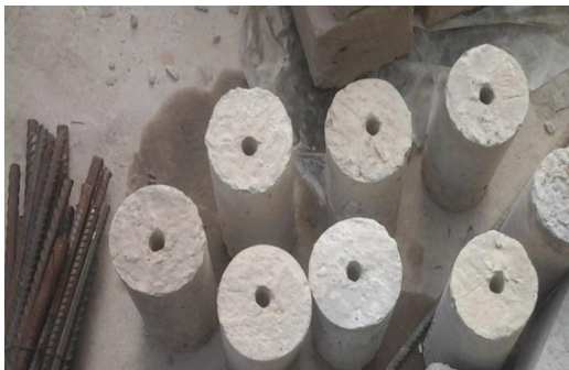
Figure 3a: Holes drilled in concrete cylinders
