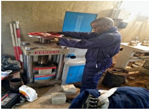
Fig. 2: Compressive strength test machine
