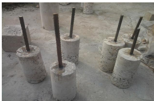
Figure 3b: Reinforcements installed using epoxy-based adhesives as binding agents.
