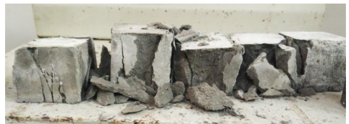
Fig 6. Broken mortar specimens after compressive test
