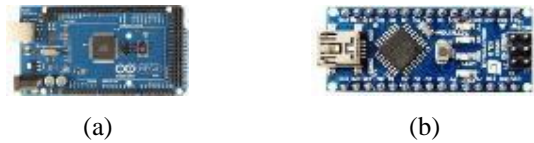
Figure 3. Microcontrollers: (a) Arduino Mega.; (b) Arduino Nano.
