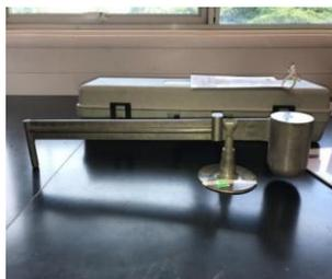
**Figure 2:** Mud density balance in pound per gallon (ppg).
