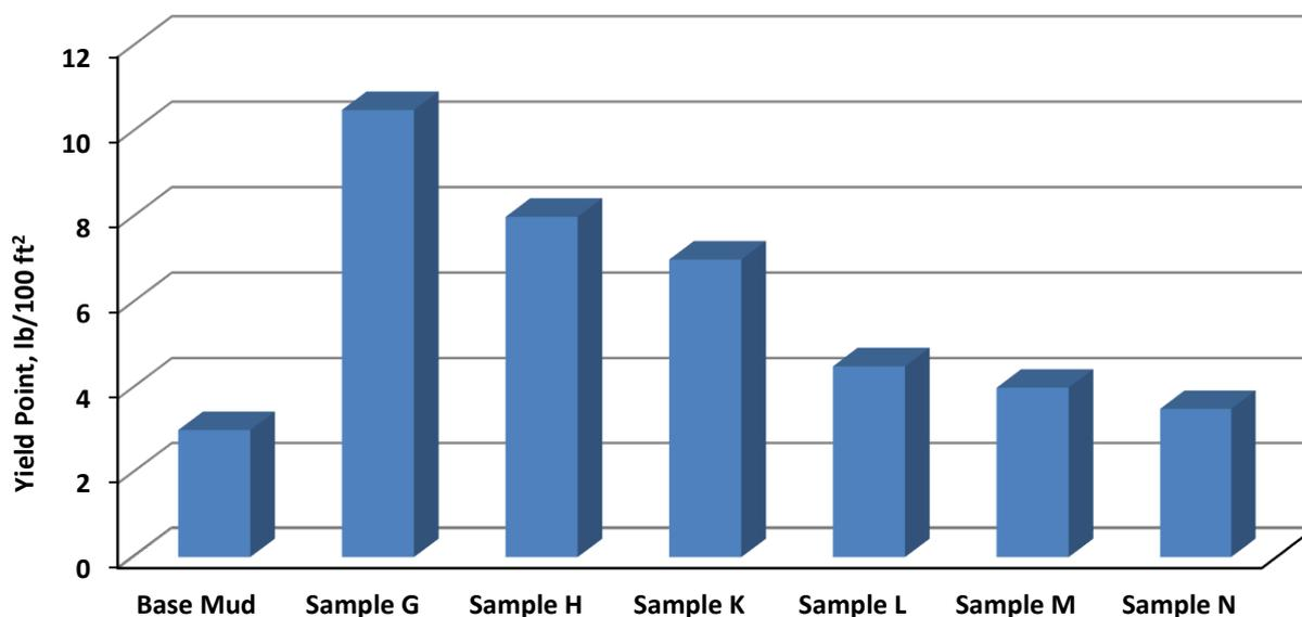
**Figure 12:** YP of WBM at different sodium bicarbonate and treating agent concentrations.
