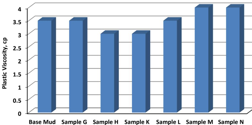
**Figure 10:** PV of contaminated and treated samples by bicarbonate and sodium hydroxide.
