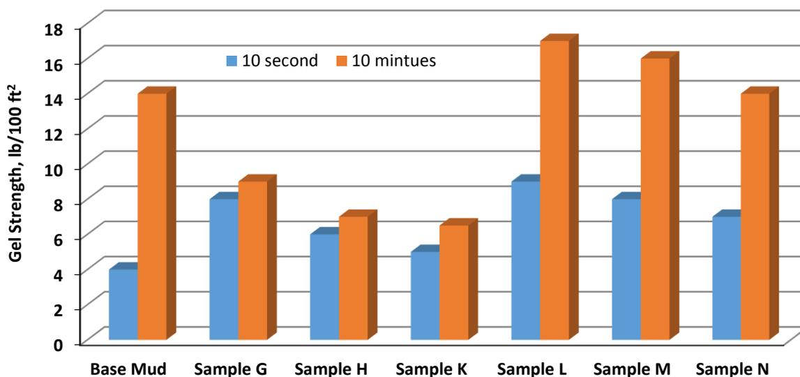
**Figure 14:** GS of fluid mud at different sodium bicarbonate and sodium hydroxide concentrations at different time.
