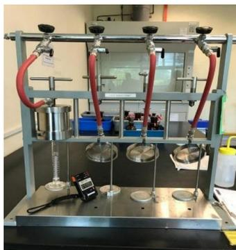
**Figure 4:** API filter press to measure mud filter loss and thickness of mud cake
