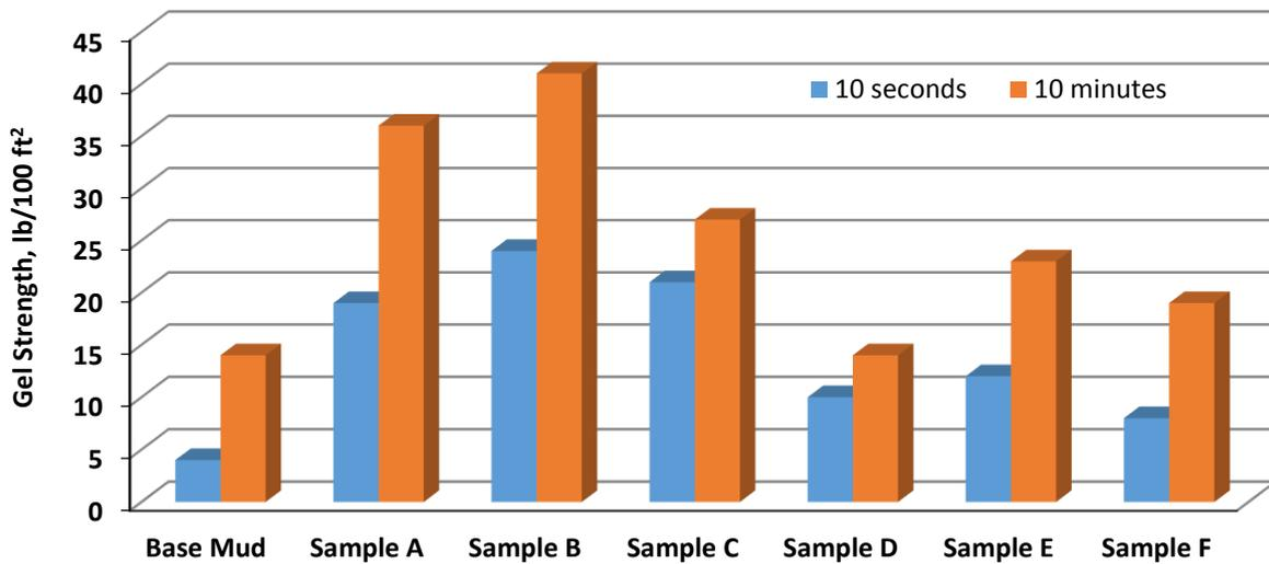
**Figure 13:** GS of fluid mud at different sodium carbonate and calcium sulphate concentrations at different time
