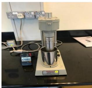
**Figure 3:** 6-speed Fann viscometer to measure mud viscosity in cP.
