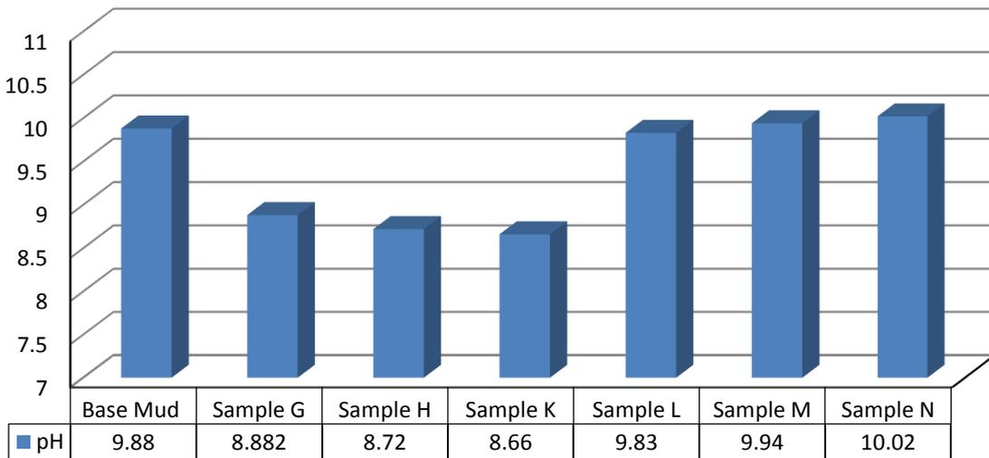
**Figure 8:** pH of contaminated and treated samples with sodium bicarbonate and sodium hydroxide.
