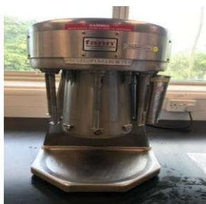
**Figure 3:** Hamilton mud mixer used to stir mud before each experiment.
