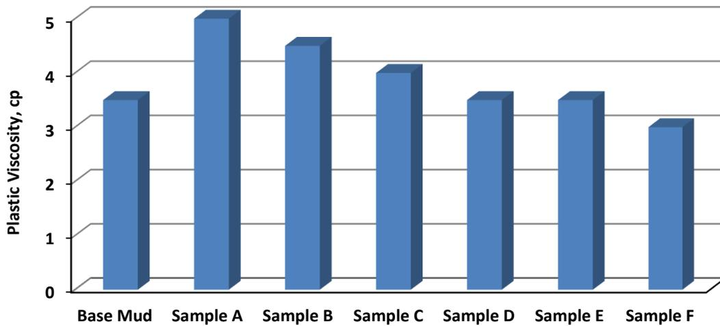
**Figure 9:** PV of contaminated and treated samples by sodium carbonate and calcium sulphate.
