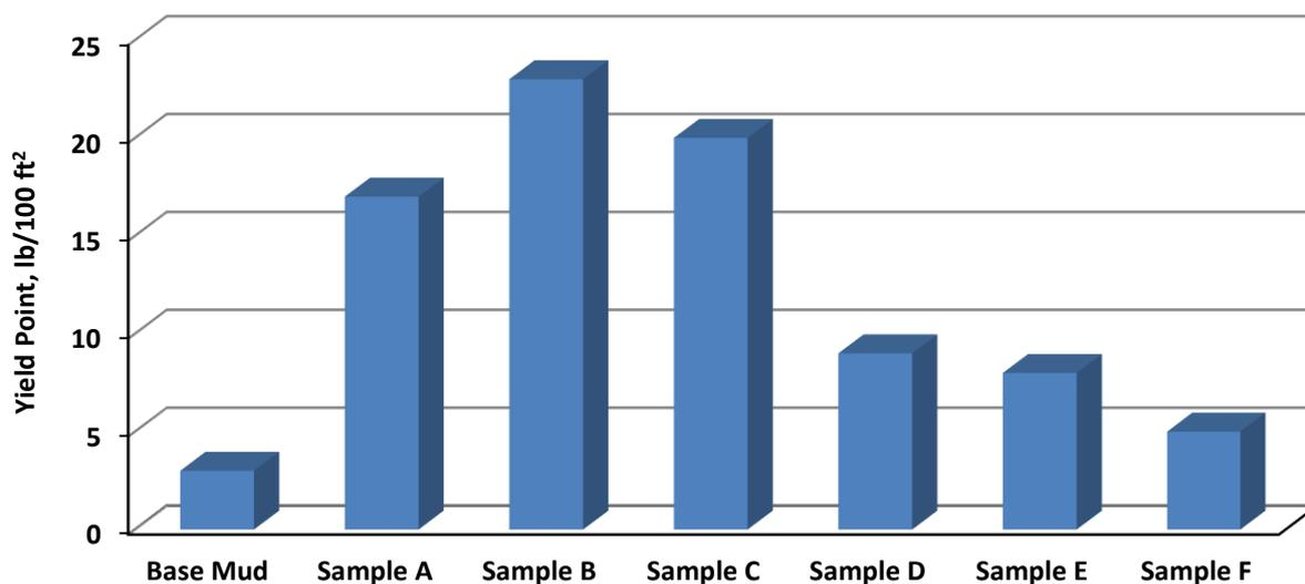
**Figure 11:** YP of WBM at different sodium carbonate and treating agent concentrations.
