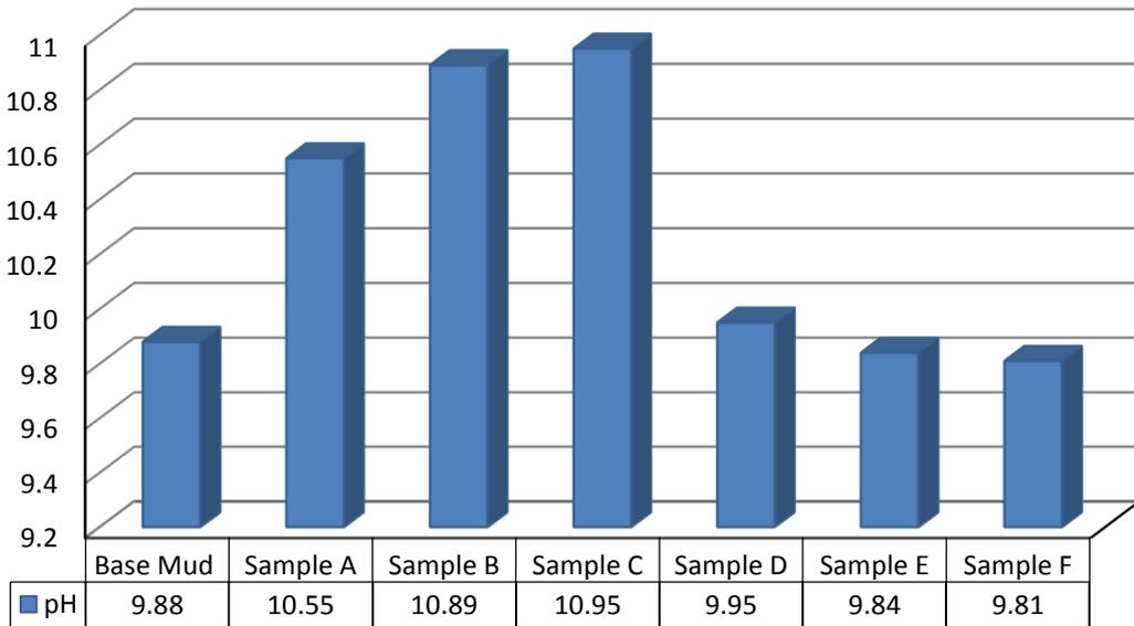
**Figure 7:** pH of contaminated and treated samples with sodium carbonate and calcium sulphate.
