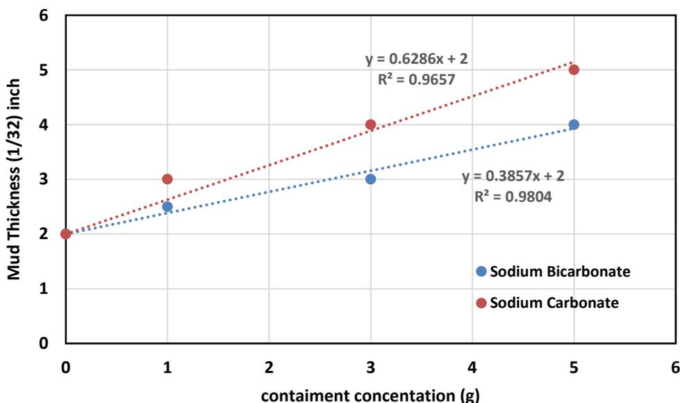
**Figure 6:** Thickness of WBM different contamination concentration
