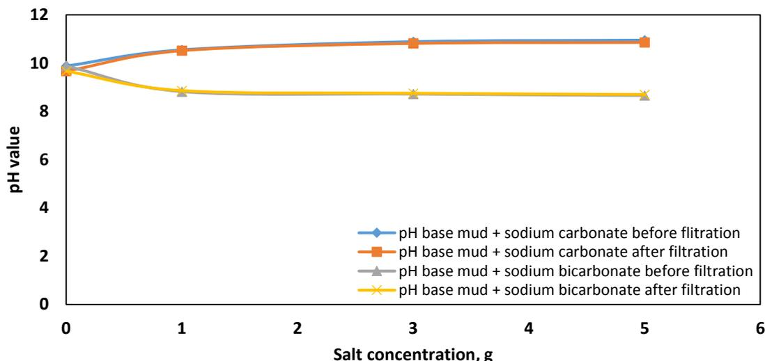
Figure 6: pH value of BM with Sodium Carbonate and Biocarbonate
