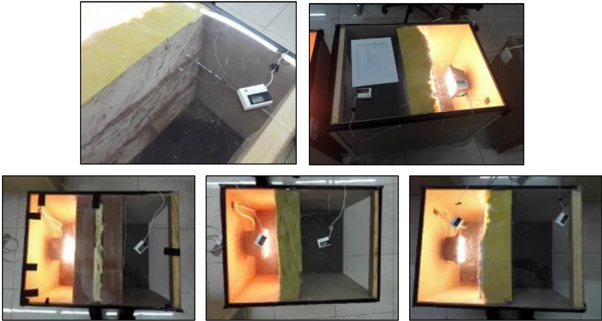
Fig 8: The three wall sections during the experiments
