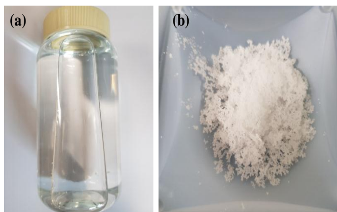
Fig. 4. Lithium carbonate in distilled water (a) and power form of lithium carbonate after drying (b)
