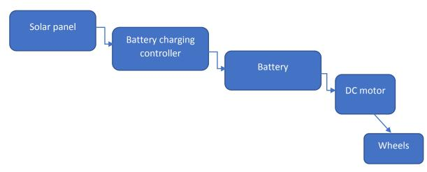
Figure 2: Block diagram of solar-powered wheelchair connection
