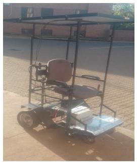
Figure 3: Solar-powered wheelchair
