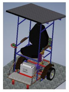
Figure 1: Design of solar-powered wheelchair
