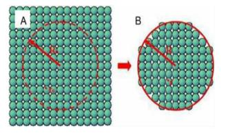
**Fig.1** A perfect crystal (A) and a nanoparticle taken out of it (B). (A) All the atoms are located at their equilibrium lattice positions. The atomic radius is r0 and the density is  $\rho$ 0. (B) The particle radius is compressed from R0 to R, the average gyration radius reduces to r, and the average density increases to  $\rho$ R. (Image curtesy from Xiaohua Yu and Zhaolin Zhan)
