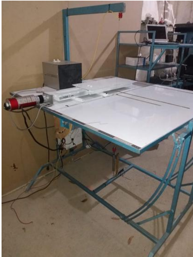
Fig. 13. Functional prototype of the hot wire cutting machine.
