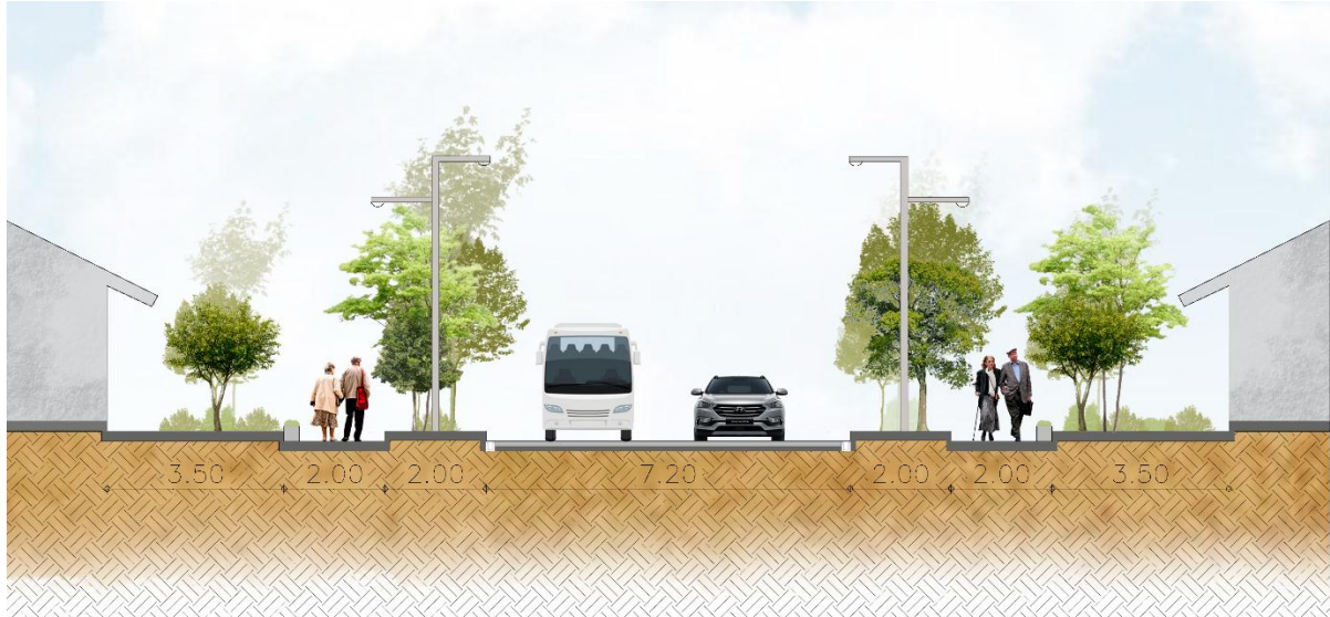
Fig. 2. Cross section of collector tracks
