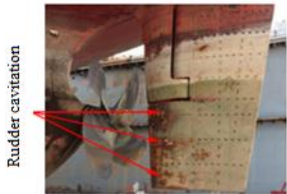
Figure 1: Illustrating cavity spots on the rudder (rudder of M/V TAN CANG FOUNDATION in periodical repair at Ship Marine shipyard, May 2017)
