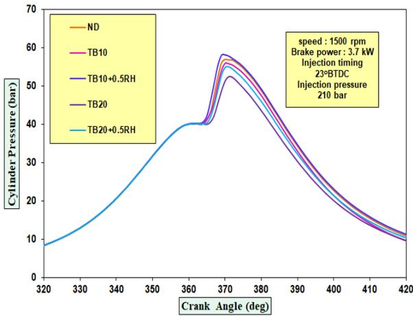
Fig. 10 Variation of cylinder pressure with crank Angle
