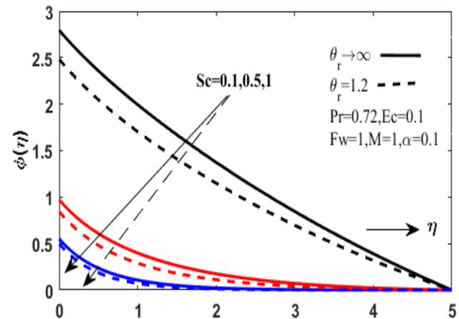
**Figure 13.** The concentration distribution for different values of  $Sc$  and  $\theta_r$ .
