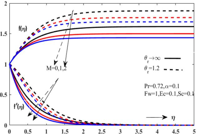
**Figure 2.** The velocity distribution for different values of M and  $\theta_r$ .
