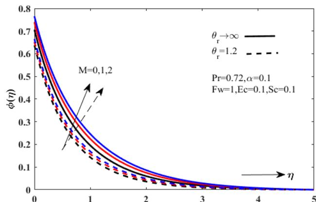
**Figure 4.** The concentration distribution for different values of M and  $\theta_r$ .
