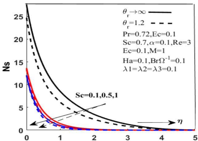
Figure 21. The Entropy generation for different values of  $Sc$  and  $\theta_r$ .
