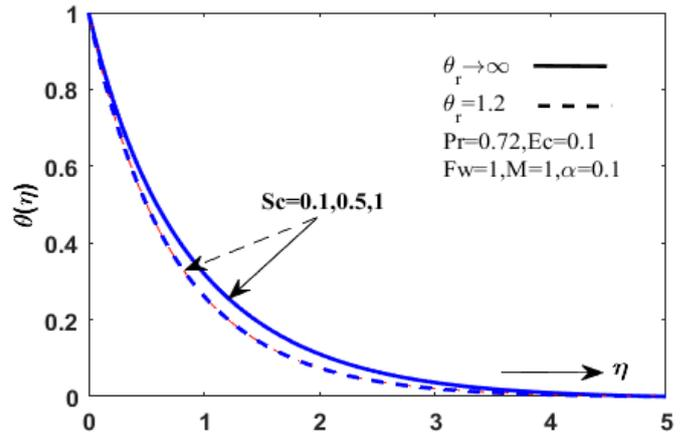
**Figure 12.** The temperature distribution for different values of  $Sc$  and  $\theta_r$ .
