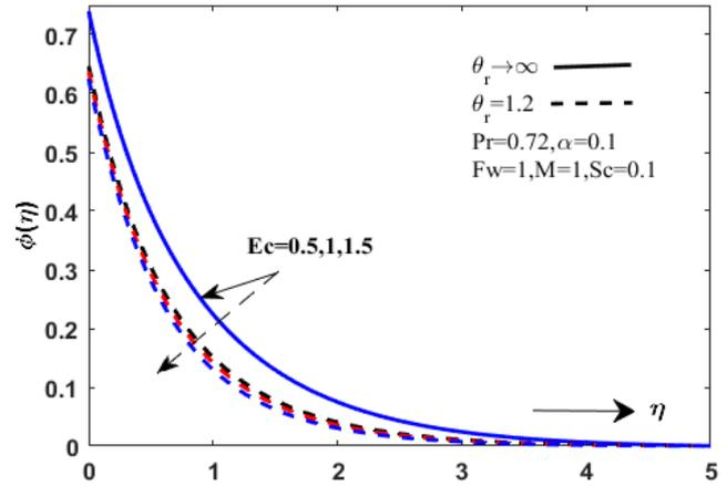
**Figure 7.** The concentration distribution for different values of  $E_c$  and  $\theta_r$ .
