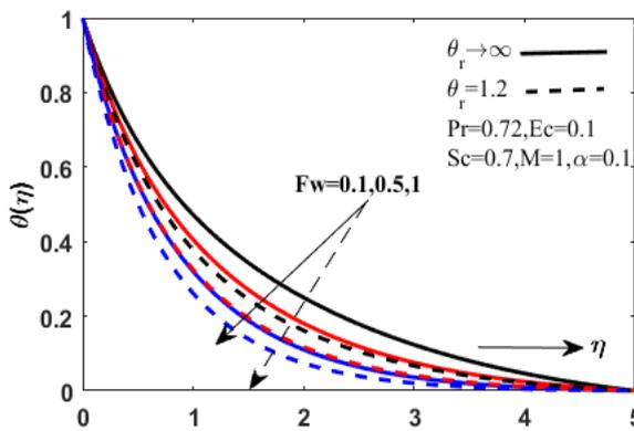
**Figure 15.** The temperature distribution for different values of  $F_w$  and  $\theta_r$ .
