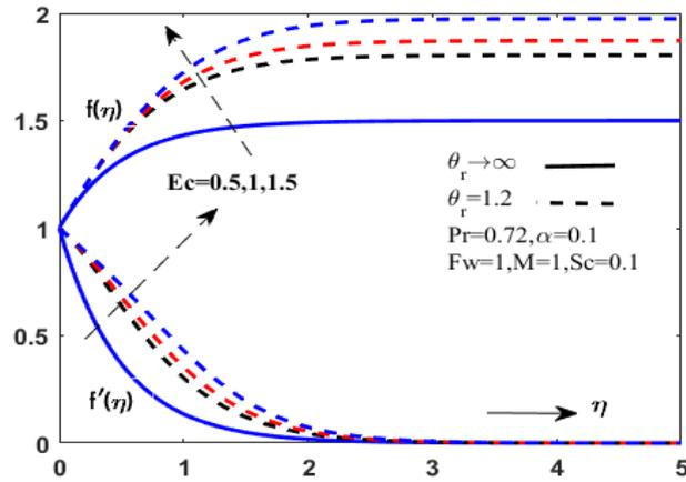
**Figure 5.** The velocity distribution for different values of  $E_c$  and  $\theta_r$ .
