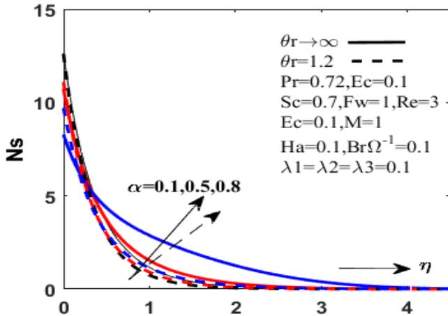
Figure 19. The Entropy generation for different values of  $\alpha$  and  $\theta_r$ .
