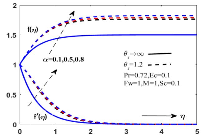
**Figure 8.** The velocity distribution for different values of  $\alpha$  and  $\theta_r$ .
