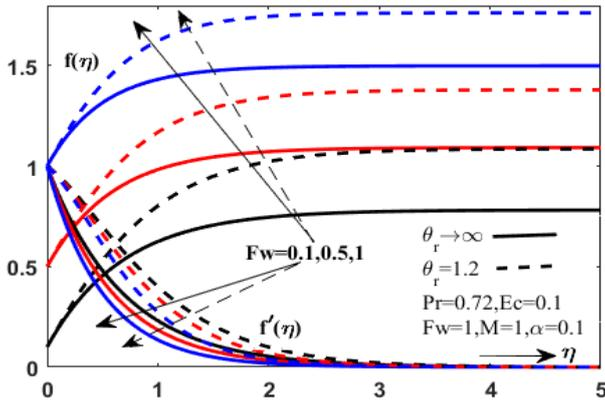
**Figure 14.** The velocity distribution for different values of  $F_w$  and  $\theta_r$ .
