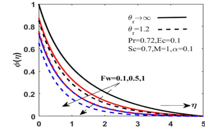
**Figure 16.** The concentration distribution for different values of  $F_w$  and  $\theta_r$ .
