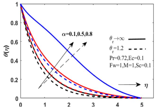
**Figure 9.** The temperature distribution for different values of  $\alpha$  and  $\theta_r$ .
