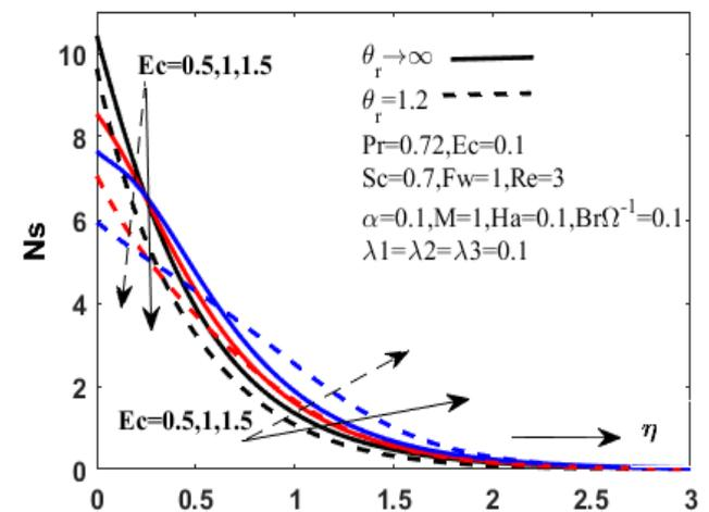
**Figure 18.** The Entropy generation for different values of  $Ec$  and  $\theta_r$ .
