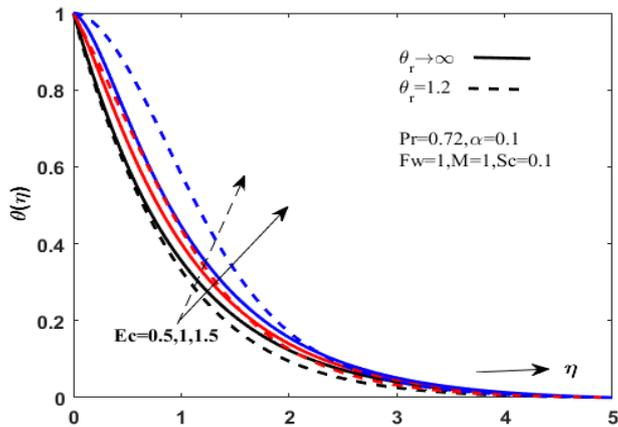
**Figure 6.** The temperature distribution for different values of  $E_c$  and  $\theta_r$ .
