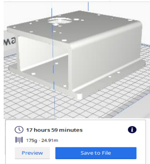
Fig. 7. 3D printing duration of X-axis part.
